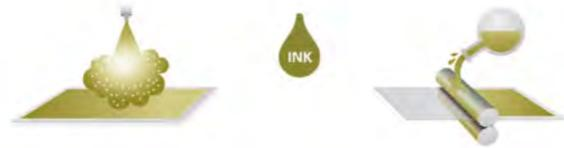
nanograde ink is printed via slot-dye, ink jet, doctor-blading etc.
